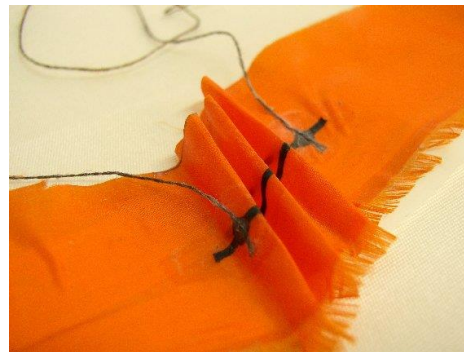
Sensor on polyamide 66 fabric
