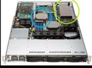
**CPUs and C1060s in workstation have active fans for airflow**
