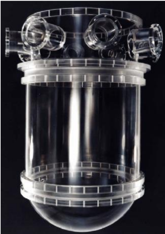
1:5 scale primary circuit of a KONVOI reactor
