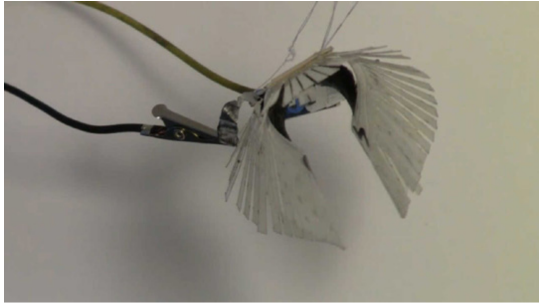
Electrical pressure on the elastomer results in the actuation of the minimum energy structures
