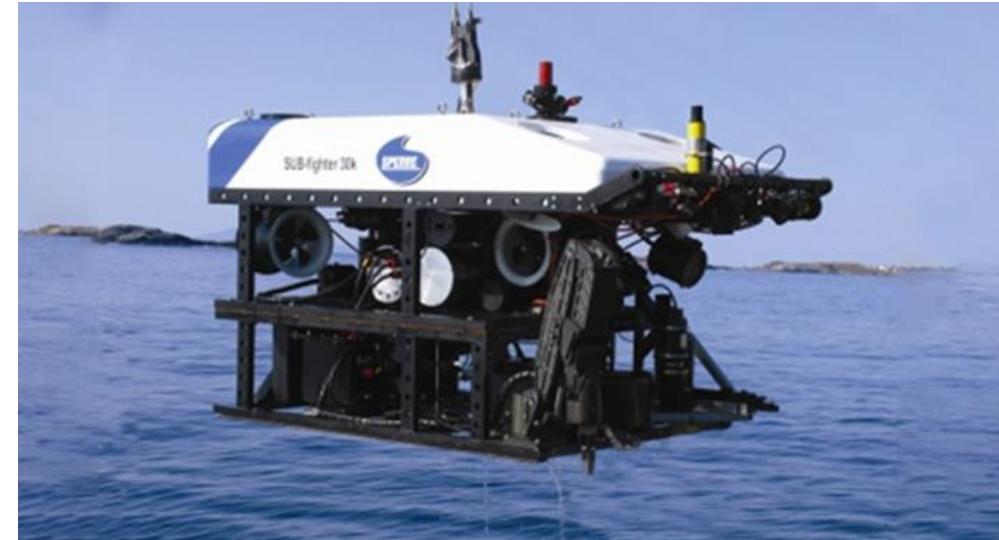
Seabed robot dedicated to submarine ore collecting
